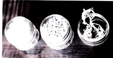
A cycle: (from left) Crushed plastic bottles, which are turned into plastic pellets and made into yarn.
